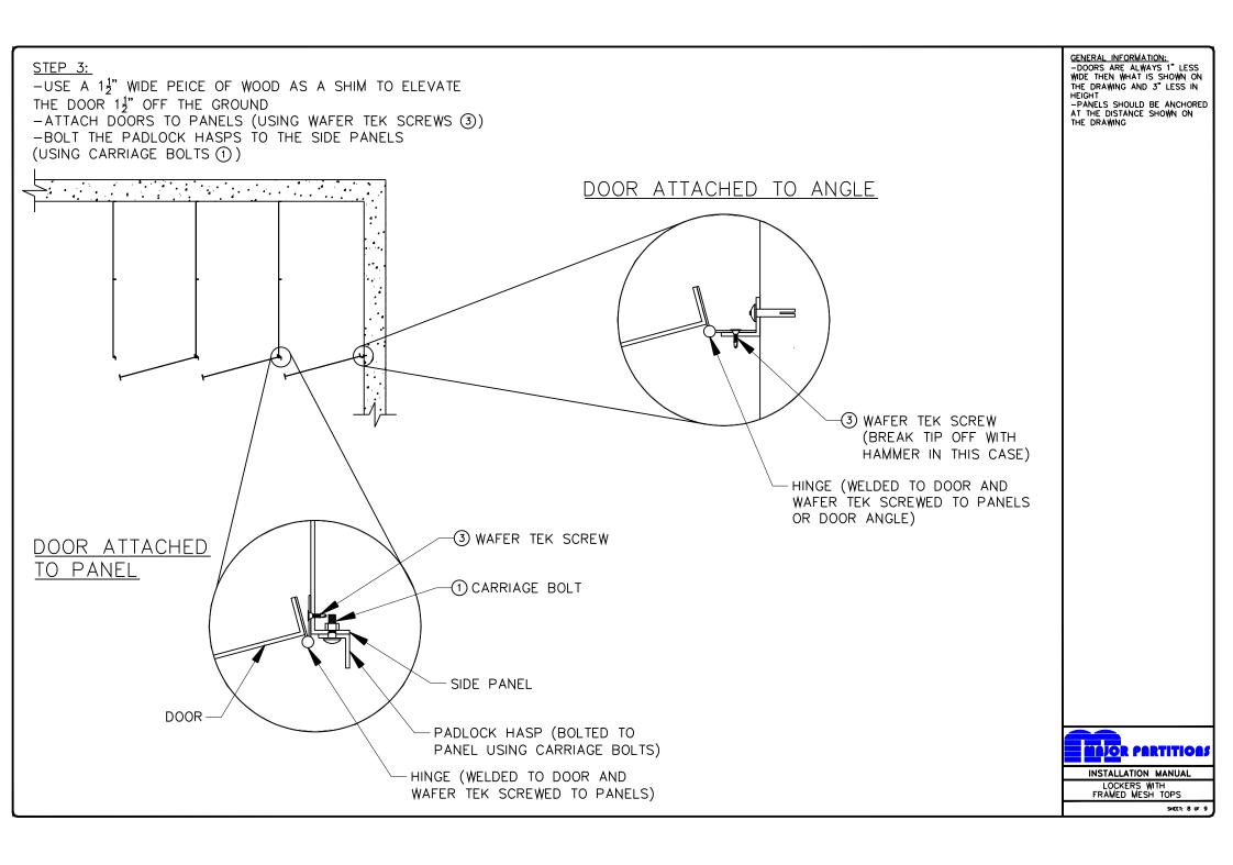
LOCKERS WITH BACK PANELS: -ATTACH PANELS TOGETHER AS SHOWN USING  $\frac{1}{4}$ " $\times \frac{3}{4}$ " CARRIAGE BOLTS (1), TEK SCREWS (2) AND CORNER BRACKETS GENERAL INFORMATION:
